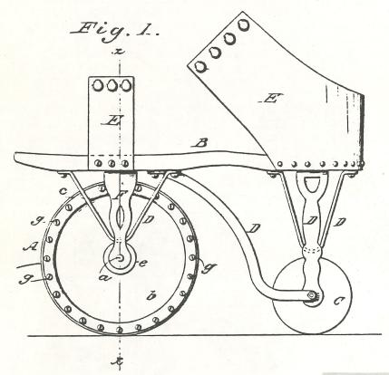
This roller skate was patented by E.F. Johnson on July 8, 1884. Similar in design to the Spaulding skate on the next page, the wheels on this skate were rubber, with leather for better traction. A lever which runs from the front truck to the rear wheel allows the latter to turn slightly. It is not known whether this 2 wheel model ever went into production.
